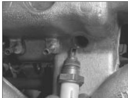
14.44 Removing the intake air temperature sensor from the rear of the inlet manifold (Zetec engine shown)
