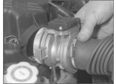
4.2c . . . and withdraw the sensor
