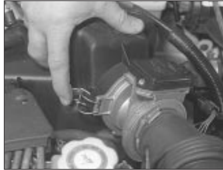
4.2b . . . release the retaining clips . . .
