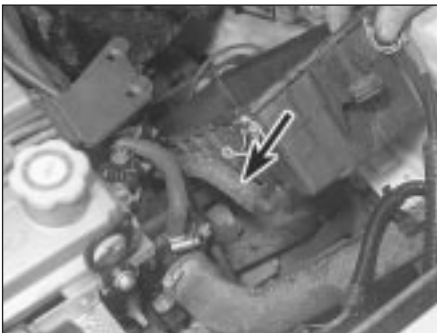
4.4 Unscrew front retaining nut and lift the air cleaner housing, disconnecting the breather hose (arrowed)
