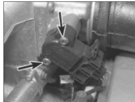
14.46 Throttle position sensor mounting screws (arrowed)
