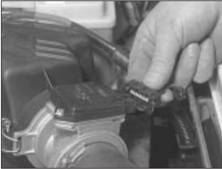
4.2a Disconnect the mass air flow sensor wiring multi-plug . . .
